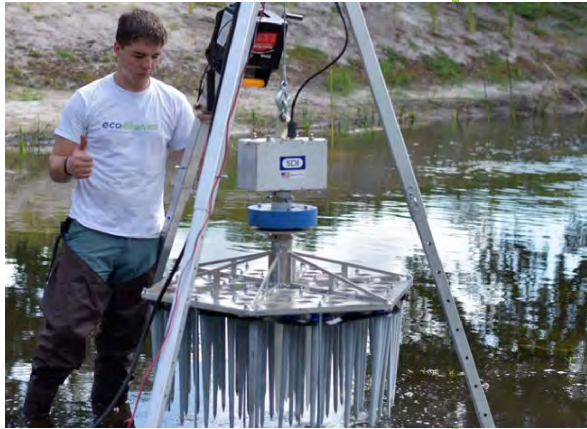
SPEARS for Contaminated Sediment
